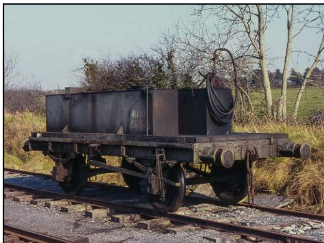
Pictured on Friday 23 March 1973 at Attymon Junction was fuel tank wagon, 406A. This wagon was used to top-up the branch locomotive so as to avoid working to Galway for refueling.
